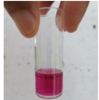
Fig. 10 – 2 ppm of chlorine at the end of the system
